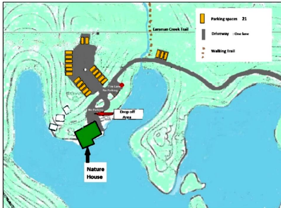
Figure 5.1: High-Level Concept of On-Site Parking Area Expansion
